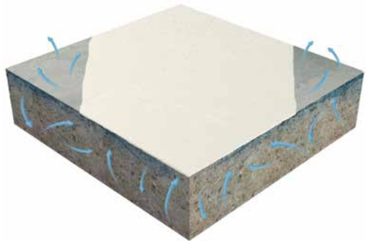
Principle of effective concrete floor curing. Curing membrane reduces the water evaporation in the early-aged concrete slab.
