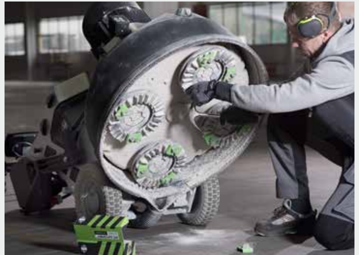
Operator changing metal bond diamond tools under an HTC DURATIQ grinding machine. The green Superprep tooling series is specifically developed for heavy preparation works.
