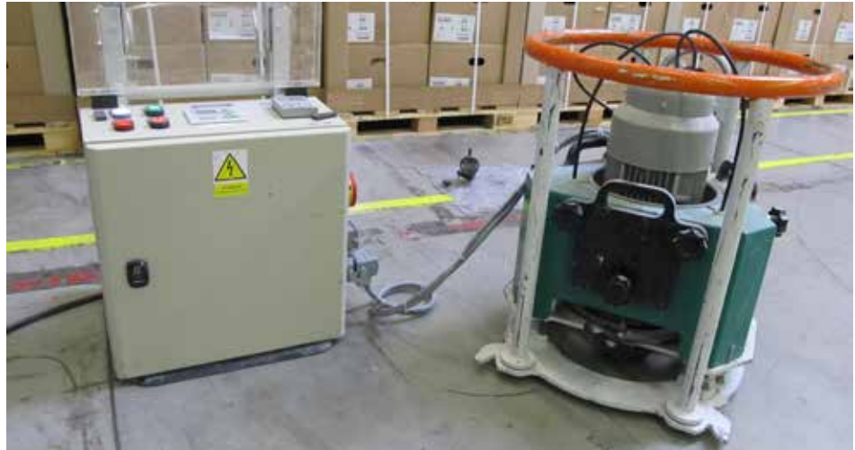
The BCA concrete floor wear resistance test equipment according to EN 13892-4.
