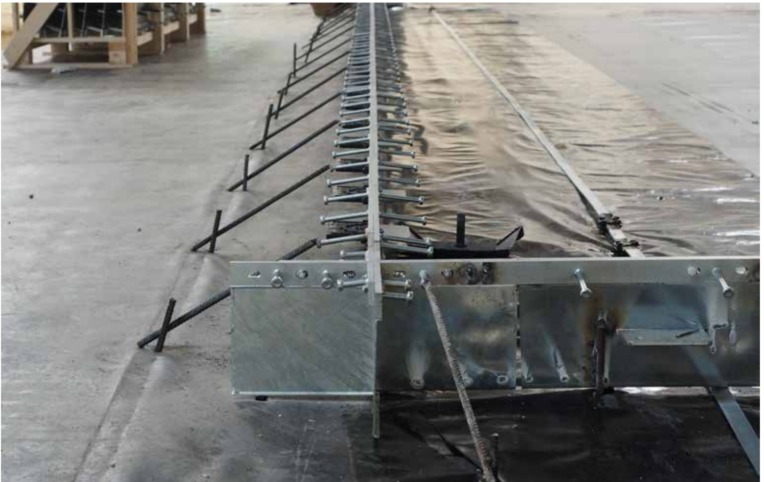
Free movement joint solution from Peikko® Group. TERAJOINT® is a prefabricated leave-in-place joint system designed to build formed free-movement joints, consisting of heavy-duty arris armoring, permanent formwork and a load transfer system. It is suitable for all large-area construction methods on ground-bearing and pile-supported concrete floors.
