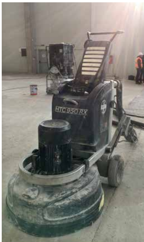
SikaScreed® HardTop-60 system requires profiled substrate. Concrete substrate was profiled accordingly by using an HTC grinding machine equipped with its special bush hammering tool "HTC Ravage".
