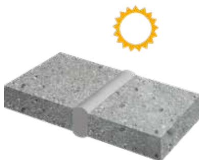
Expansion of building elements
